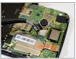
• Disconnect the marked connector with a pair of tweezers and remove the camera piece.
