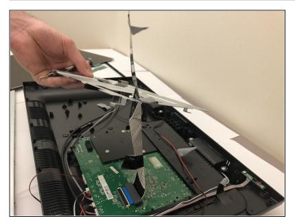
The rectangular piece will still be attached to the motherboard beneath it with a strip of tape. Remove this strip of tape.
