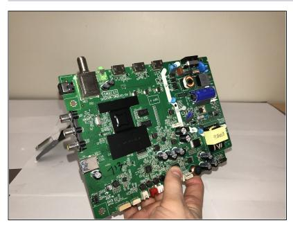
• After removing the nut from the cable input, the black plastic should easily slide off of the inputs on the board. There are two separate pieces of plastic on the board, so be sure to remove both.
