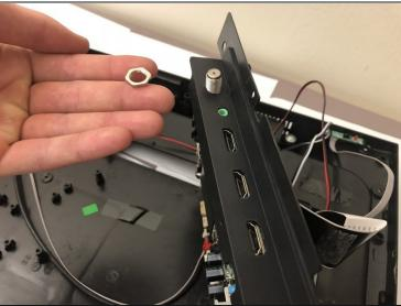
• After following the prerequisite guides, you should have the main board off with the black plastic still on. To remove the plastic, unscrew the nut that holds this plastic to the cable input on the board.
