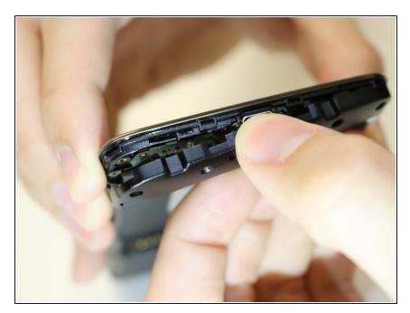
Remove the plastic casing on the bottom of the phone by gently pulling.
