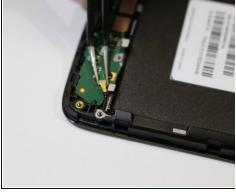
Remove the three connectors on the board below the battery slow by gently pulling on the small gold tab with a pair of tweezers.
