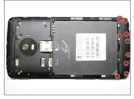
Remove the nine (9) 4mm Philips screws securing the daughterboard cover.
