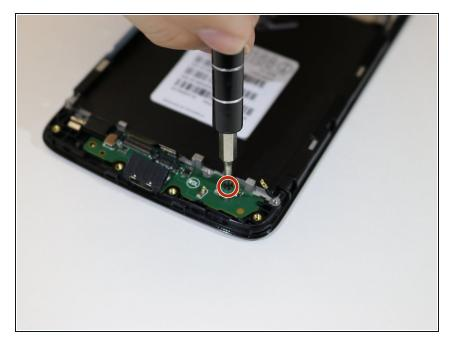
Remove the 3.4 mm Philips screw securing the daughterboard to the frame.
