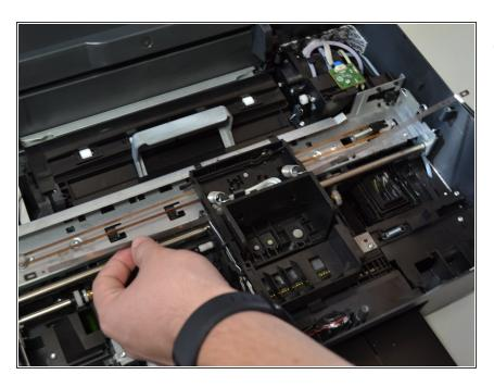
Carefully slide the encoder strip out from the carriage.
