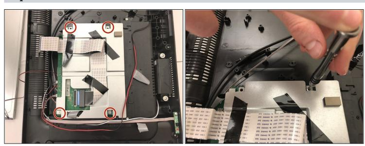
• Unscrew the four screws surrounding the steel rectangle with a Phillips 00 Screwdriver.
