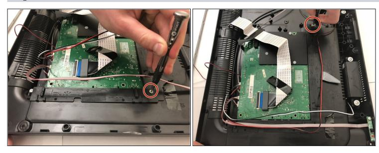
• Use a Phillips #00 screwdriver to remove the two screws on both sides of the motherboard.
