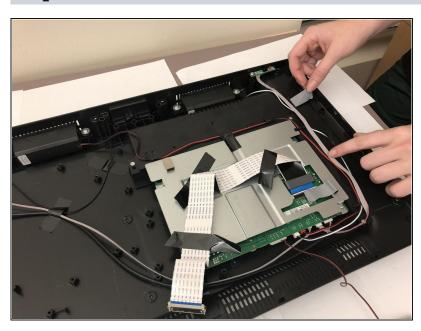
Remove all strips of tape attached to the silver steel rectangular piece.
