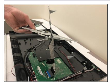
• The rectangular piece will still be attached to the motherboard beneath it with a strip of tape. Remove this strip of tape.
