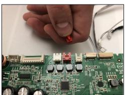
• Remove the remaining three wires from the mainboard.
