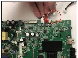
• There are 5 wires attached to the motherboard. Remove the two thicker white wires to the right of the red wire.
