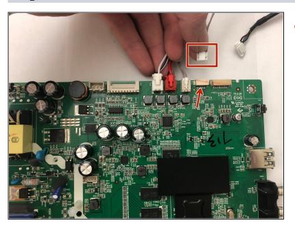
Plug the new sensor's cable into the motherboard. Make sure to plug it into the correct location.
