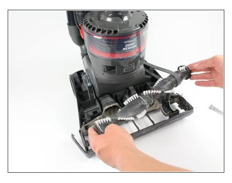
Grab on both ends of the roller brush, lifting it and the attached belt clear of the housing.
