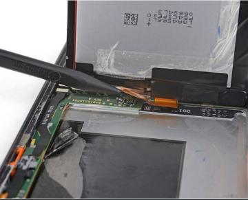
Use the tip of a spudger to lift the battery connector up out of its socket on the motherboard.
