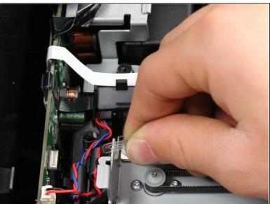
Pull the encoder strip toward the slot it rests on to relieve the tension on the hook and slide the strip off the hook.
