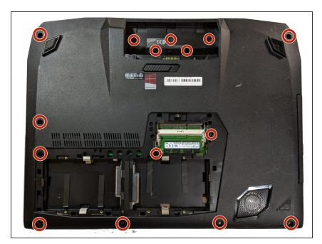
Remove the 8.5mm screws holding the bottom half of the laptop together.
