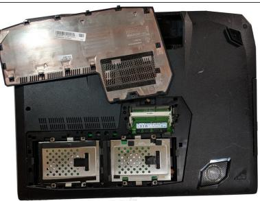
Once the screw is out, pull on the plastic tab to pull off the plastic cover.
