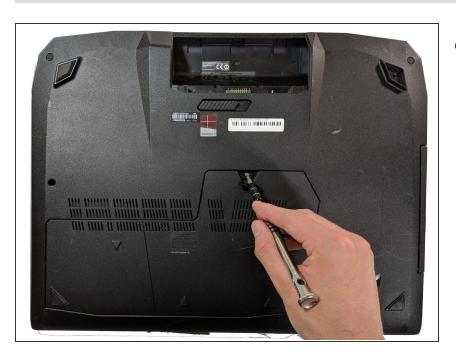
Unscrew the 5.2mm screw underneath the flap.
