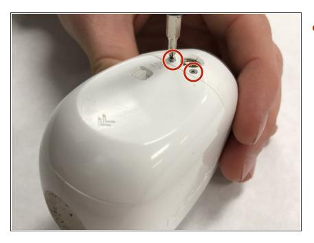
Remove the 2 (3.5mm) housing screws with a J0 screwdriver.
