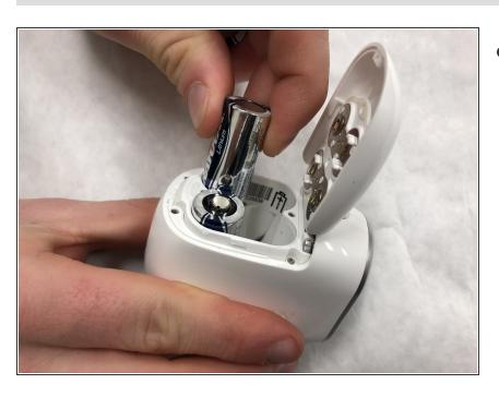
Remove all 4 of the 3.0 Volt batteries from the battery housing.
