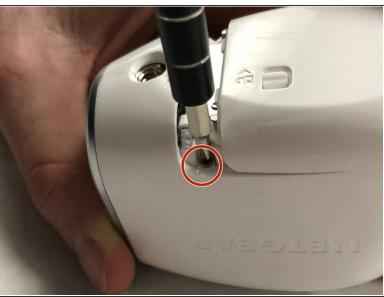
• Slide the unlocked battery cover forward to remove 2 (3.5mm) screws, that are behind the cover.
