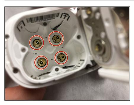
Inspect prongs at the bottom of the battery housing to ensure that they are not bent or broken before replacing the batteries.
