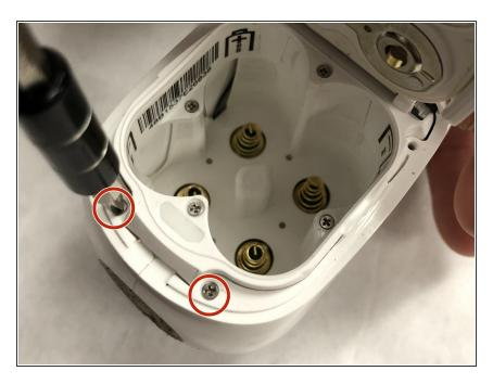
Open the battery cover and remove the 2 (3.5mm") screws from under the cover.
