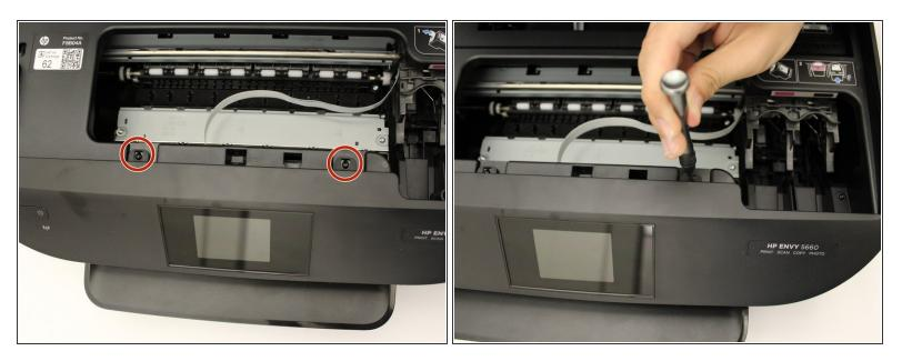
Remove the two 12 mm screws with a T10 bit.
