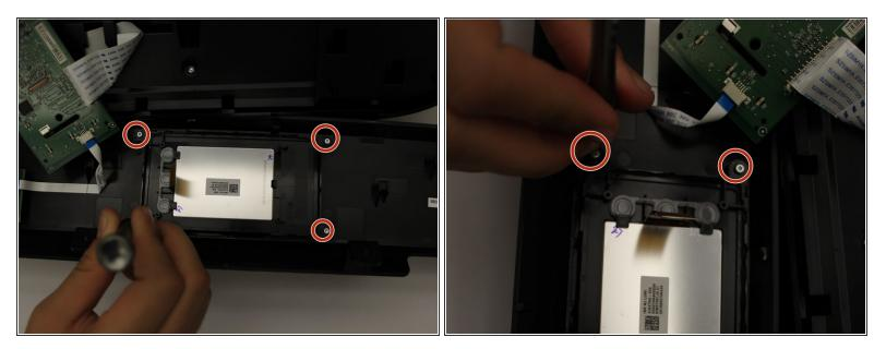
• Remove the four 5 mm screws with a T6 bit, allowing you to separate the LCD from the cover,
