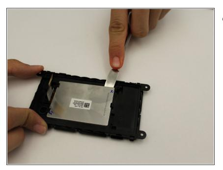
Place the metal spudger underneath the LCD and gently lift up to remove the LCD.
