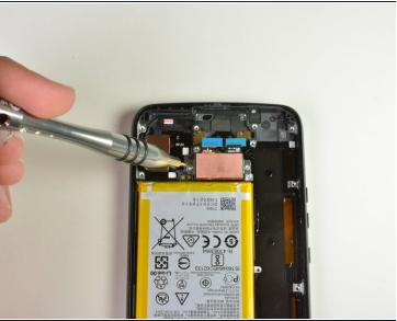
• Using a T3 Torx screwdriver, remove both 1cm screws. To do this, insert the screwdriver into the head of the screw, then turn counter-clockwise.
