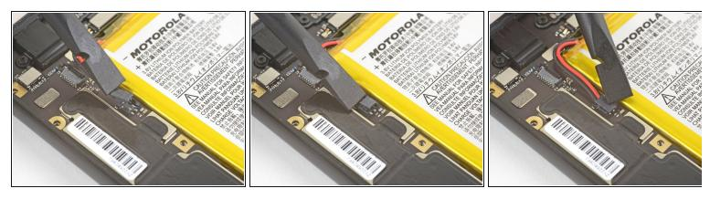
To re-connect the battery, align the connector on top of the socket, and press it down with your finger or a spudger.
