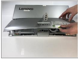
• Locate the slot on the right side of the computer next to the screw hole. Use a plastic opening tool or spudger to pry off the rear cover. (Don't be afraid to use a little force.)
