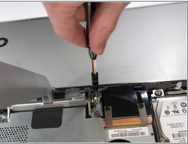
Remove the four screws that secure the arm stand.
