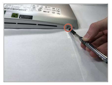
Remove the two screws on the bottom of the computer, one on each side.
