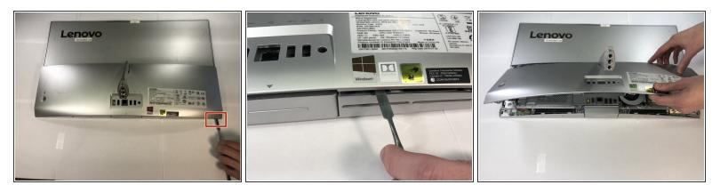
Locate the slot on the right side of the computer next to the screw hole. Use a plastic opening tool
