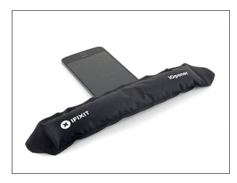
• <u>Apply a heated iOpener</u> to the top edge of the phone for at least 90 seconds.
