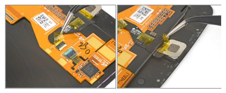
• Use tweezers to peel off any tape on the home button connector and home button
