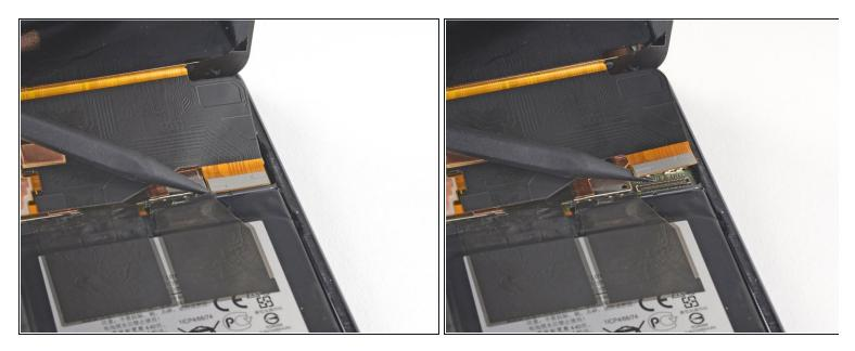
• Use the point of the spudger to lift and disconnect the display cable connector from its socket.
