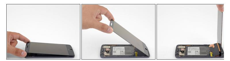
• Lift the earpiece end of the display up to provide access to the display cables.
