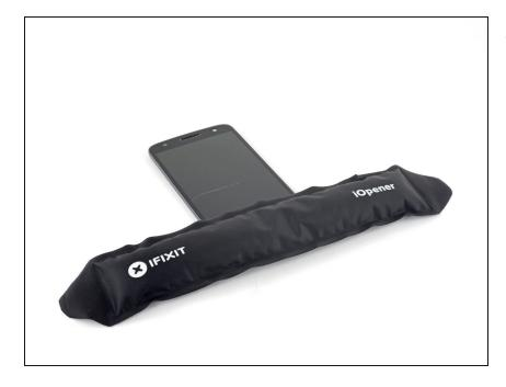
Apply a heated iOpener to the bottom edge of the phone for at least 90 seconds.
