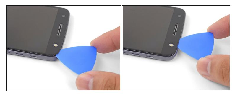
Insert an opening pick into the flash side corner of the phone and carefully slice around the flash unit.
