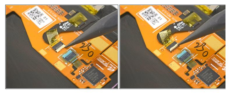
• Use the point of a spudger to flip up the home button connector's lock.
