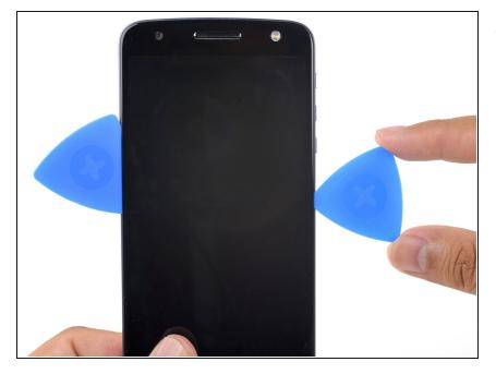
• Repeat the heating, lifting, and cutting steps for the remaining long edge of the phone.
