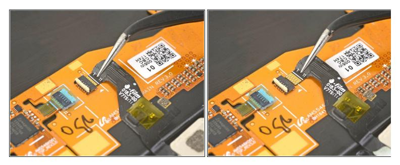
• Use tweezers to carefully pull the home button cable straight out of the socket.
