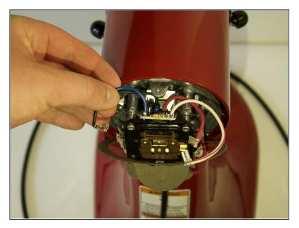
Grab the wires and tilt the edge of the board up to lift the circuit board up and out.
