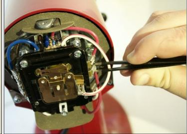
• Using pliers or <u>tweezers</u>, remove the connectors of the four wires attached to the circuit board.
