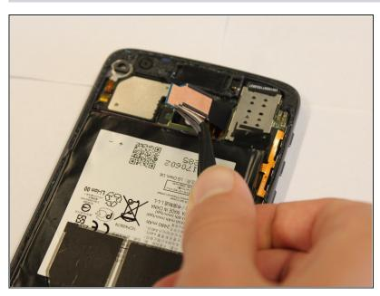
Slowly and carefully lift up on the tab until it pops out of the phone and is only connected by the black tape.
