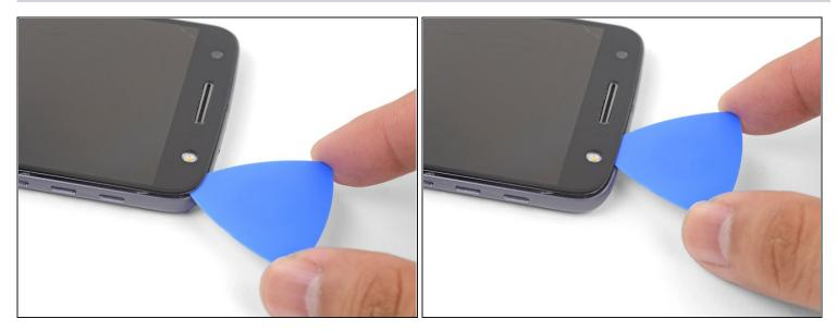
• Insert an opening pick into the flash side corner of the phone and carefully slice around the flash unit.
