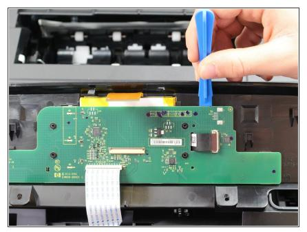
the space between the green board and the printer manifold and push downwards to dislodge the green board.
