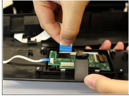
Remove the connector that is attached to the screen's circuit board by pinching the blue part of the connector with two fingers and pulling it away from the circuit board.
