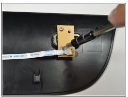
Using the Torx T6 hex screwdriver, remove the 7.0mm screw that binds the front cover to the printer body by turning the screw counterclockwise.
