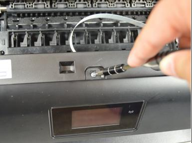
Using the 2.0 mm hex screwdriver, remove the 14 mm hex screw that binds the front cover to the printer body by turning the screw counterclockwise.
