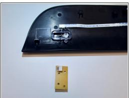
• Remove the connector that is attached to the screen's circuit board by pinching the blue part of the connector with two fingers and pulling it away from button circuit board.
