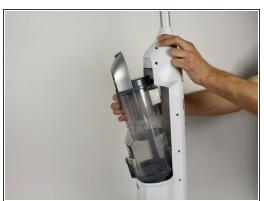
Push the grey button on top of the dust cup canister and pull the canister off at the same time.
