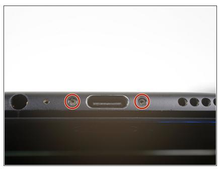
Remove the two 2.6 mm T2 screws straddling the USB-C port on the bottom edge of the phone.
