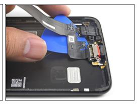
Slide an opening pick underneath the port assembly's flex cable to loosen it from the back cover.
