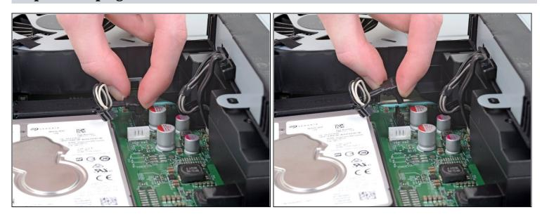
Unplug the SATA cable connecting the hard drive to the motherboard by pulling directly upward.
