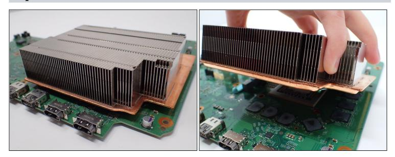
• Lift the heat sink to detach it from the motherboard.
