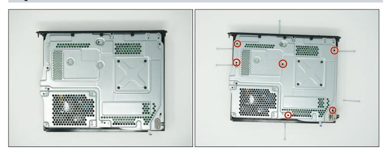
• Use a Torx T9 screwdriver to remove the six 47mm long screws, which attach the bottom side of the outer case.
