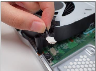
• Disconnect the plastic wire connector from the motherboard.
