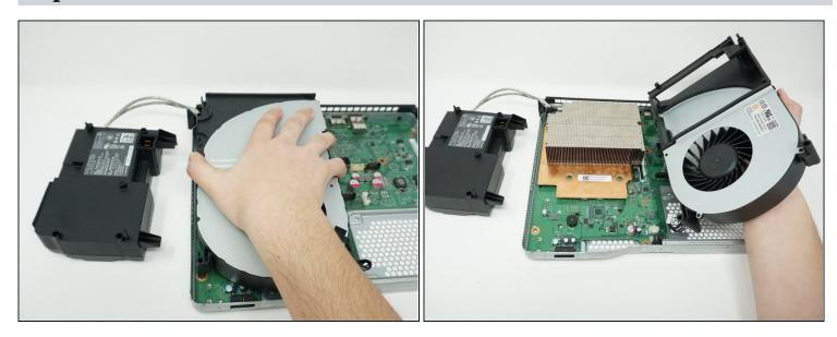
• Remove the cooling system by lifting it vertically off of the motherboard.
