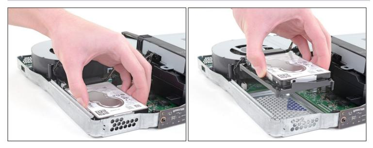
• Lift the hard drive assembly up out of the upper metal case.
