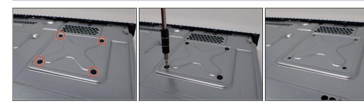
• Using a T9 Torx screwdriver, remove the four 9mm screws that are holding the heat sink to the outer metal casing.
