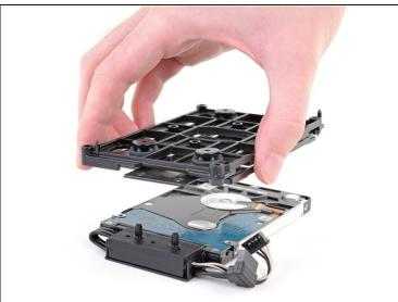
• Lift the mounting bracket off the hard drive.
