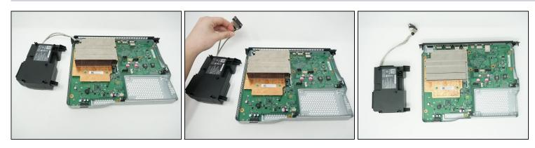
• Lift the metal piece connected to the cord out of the case.
