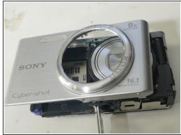
Remove side panels and then remove front cover
