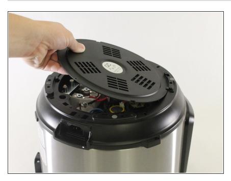
Rotate the base counter-clockwise, then gently lift the base off of the device.
