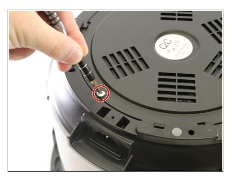
Remove the single 12mm Phillips #2 screw holding the base to the device.
