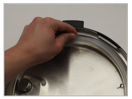
• Remove by gently pulling from the top of the sealing ring.
