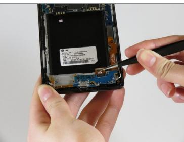
• Gently using <u>tweezers</u>, disconnect the connector that is on the bottom right.
