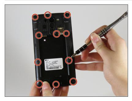
Using a Phillips #000 screwdriver, remove all eleven 3.0 mm screws from around the perimeter of the phone.
