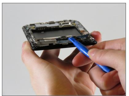
With your plastic opening tool, gently lift up the bottom edge of the exposed charging port, sliding along the edge until it lifts out.
