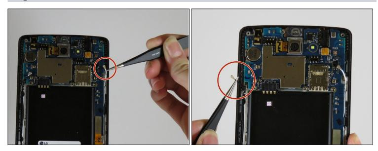
• Remove the antenna wires on both sides of the device.
