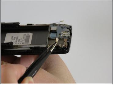
• Gently unplug the antenna wires on the bottom left and right sides of the device.
