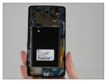
Use the same method to pry off the hard shell covering at the bottom.
