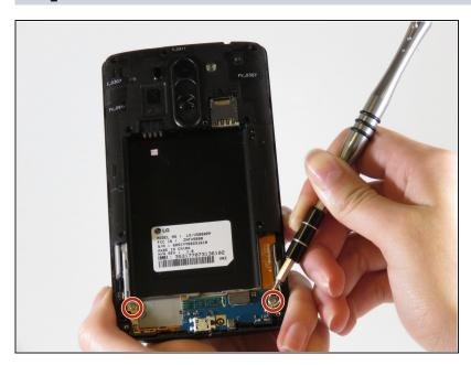
• Remove the two 1 mm Phillips #000 screws.
