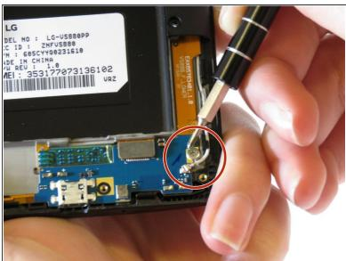
Using a Phillips #000 screwdriver, remove the two screws from the device.
