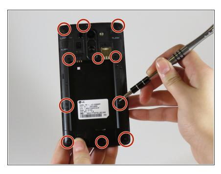
Using a Phillips #000 screwdriver, remove the eleven 3.0 mm screws around the perimeter of the phone.
