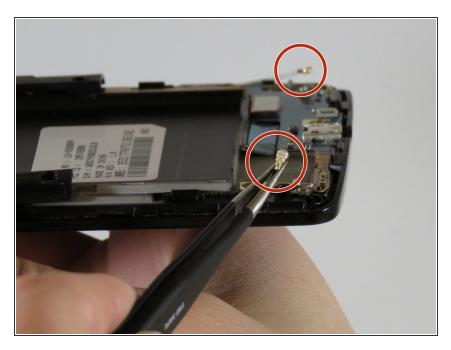
Using a pair of tweezers, lift up the two antennas surrounding the battery.
