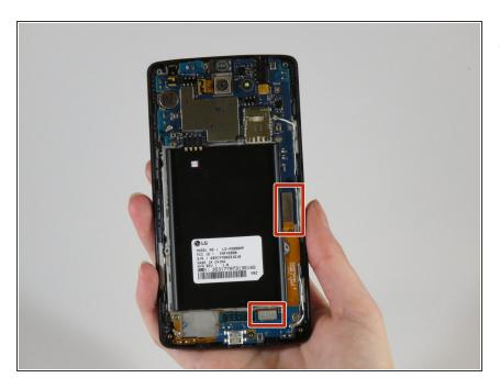
Disconnect the two connectors on the right side of the charging port.
