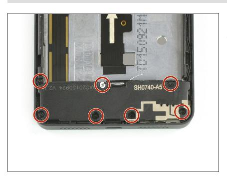
Take out the seven 4mm Phillips #00 screws, holding the loud speaker unit to the mid frame of the phone.
