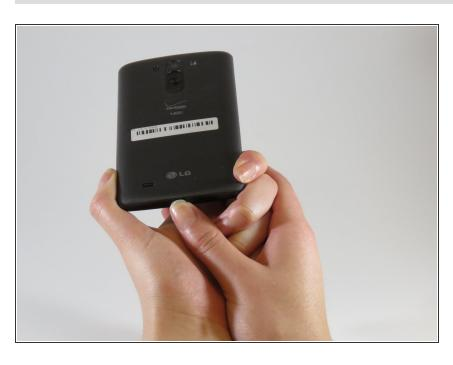
Remove the back cover by gently prying open the case of the device from the charging port.
