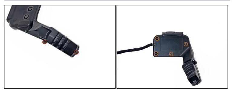
• Remove the two 7.5 mm Phillips screws on the front of the viewfinder housing.
