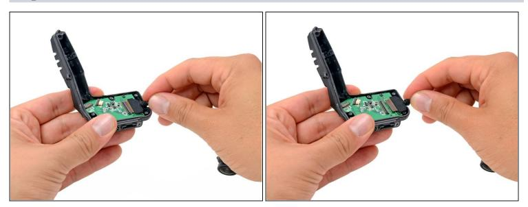
• Remove the button board data cable from its socket on the button board.
