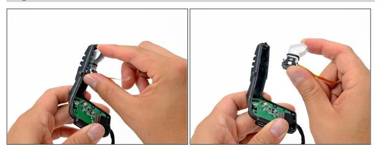
• Remove the viewfinder lens assembly from the viewfinder housing.
