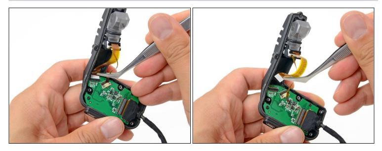
• Using your fingers or tweezers, remove the LCD ribbon cable from its connector on the button board.
