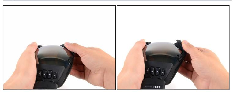
🗷 Rotate the device 180 degrees.
