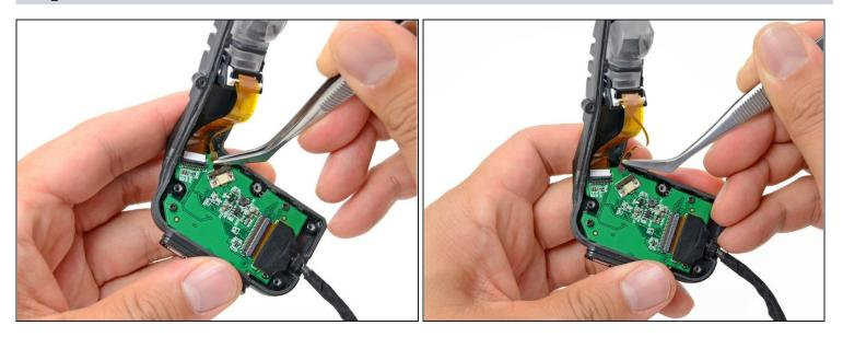
• Using your fingers or <u>tweezers</u>, gently pull out the backlight ribbon cable from its connector on the button board.
