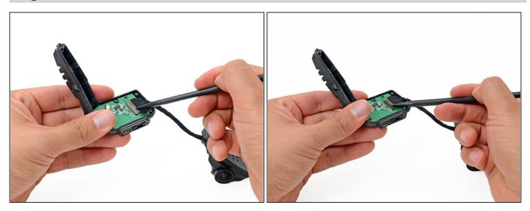
• Use the tip of a spudger to flip up the retaining flap on the button board data cable ZIF connector.
