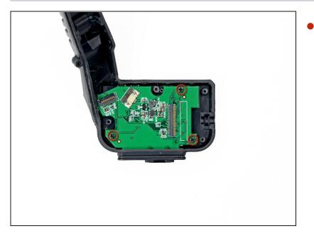
Remove the three 4.5 mm Phillips screws securing the button board to the viewfinder housing.
