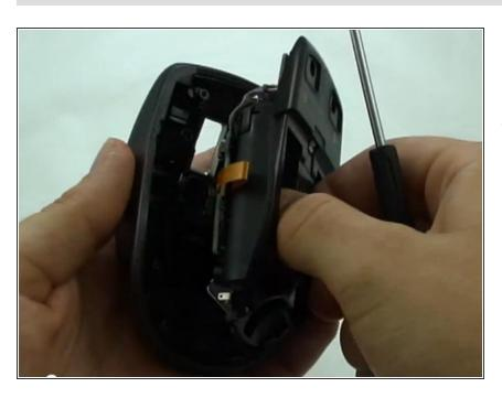
Lift the upper shell away from the base. No cable connects the two parts.
