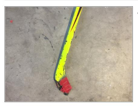
Identify a composite hockey stick with a broken blade or lower shaft. The stick must be broken below the point where the stick tapers. If it is above this point the repair is not feasible and the stick must be discarded.
