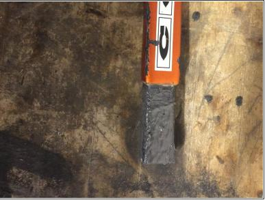
Apply glue to the portion of the replacement blade that will be inserted into the shaft. Apply enough enough to make a even coat.
