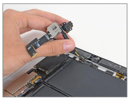
Peel the front camera and microphone cables off the rear panel.
