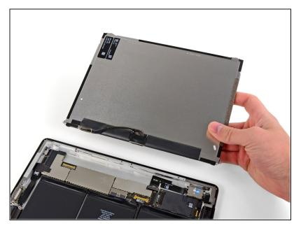
Remove the LCD assembly from the rear panel assembly.
