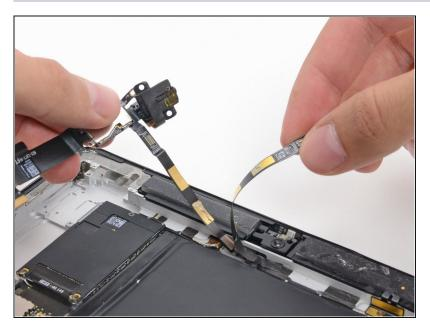
Peel the front camera cable off the microphone cable.
