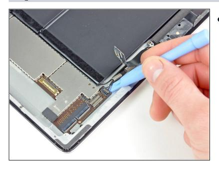
Place the prying tool beneath the 4 wires on the end of the connector and gently pry the speaker cable connector straight up from its socket on the logic board. Do not pry from the opposite end of the connector as this will break the 4 solder points on the underside of the socket and will require a microsolder repair.
