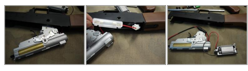
Carefully remove the gearbox from the receiver, making sure that the wires don't get stuck.
