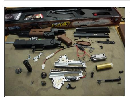
The RK47 is now fully disassembled.
