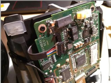
Remove the connectors plugged into the main circuit board
