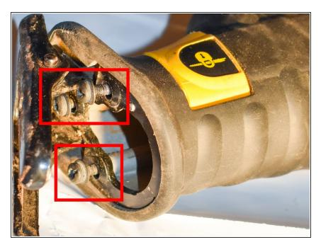
Remove the 3 screws holding the guide foot and plate to the saw body with a T20 Torx or medium flatblade screw driver.
