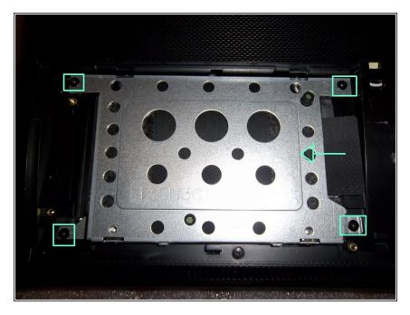
To extract the hard drive, remove 4 Ph00 screws indicated and pull the plastic tab to the left.
