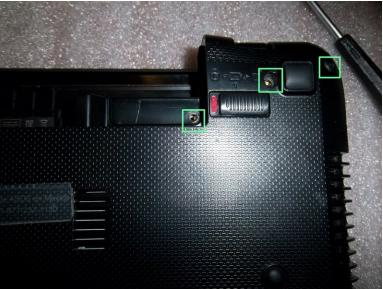
You can safely remove all the screws from both sides of the battery, they won't let the display loose.
