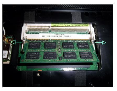
Remove the RAM module(s) by displacing both metal tabs outwards.
