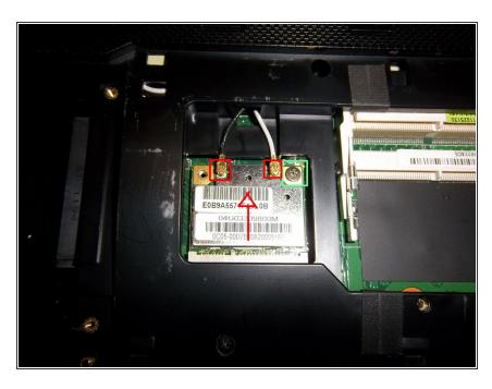
Remove one Ph00 screw to pull the Wi-Fi card, then carefully disconnect both antenna cables, mind the black and white settings.
