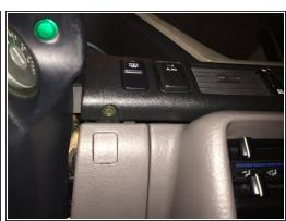
Remove the 3 screws holding the cover in place.
