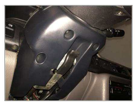
Option 1: With height adjustable steering wheel: remove the screw holding the top steering column trim and lower the column to its lowest by releasing the lever. Remove the top steering column trim.
