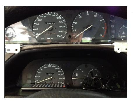
Finally: Remove the 4 screws holding the dashboard. Disconnect the 3 connectors and speed wire and you are done!
