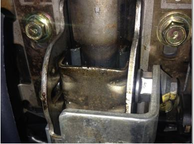
Option 2: Without height adjustable steering column: Remove all 4 screws of the steering column trim. Afterwards: remove the large golden screws. Be carefull whilst removing the last one: hold the column tight with one hand or it will fall, since it is screwed to nothing else.
