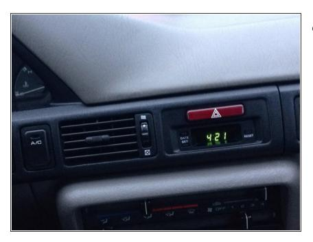
After Option 1 or 2: Pull the trim out of its holding clips. Disconnect all wires, except for clock and hazard switch. Slowly remove the trim, in case of Option 1: you might have to slightly bend the trim, be carefull. Afterwards: Rotate the trim 180° around the clock wire.
