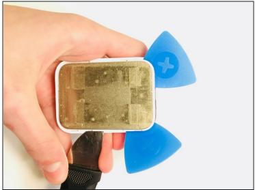
• Carefully remove the clips on the side by pushing up with the Jimmy. If needed, use the plastic Opening Picks to keep the back piece from popping back into place.
