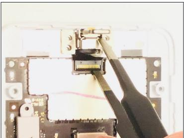
• A similar adhesive can be found covering the plug for the Lightning connector. Peel the adhesive back and gently lift the cable to disconnect the connector.
