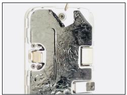
• The silver adhesive is covering two Phillips screws at opposite ends of the dock. Peel back the adhesive on these areas and remove both screws.
