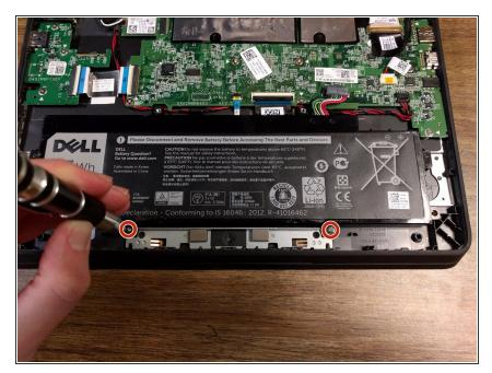
• Remove the two silver screws that hold the battery to the case
