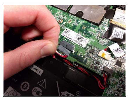
• Unplug the battery connector from the motherboard
