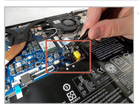
Disconnect the battery from the motherboard.
