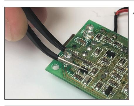
Gently pry the LEDs using one of the Precision Tweezers.
