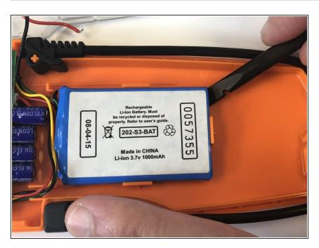
Using the spudger, pry the battery off the back cover.
