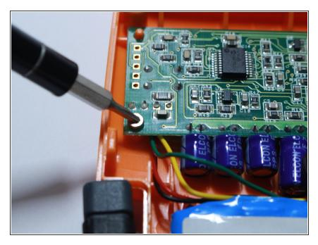
Using a T6 Torx screwdriver, unscrew the 5.66 mm screws attaching the circuit board to the case.
