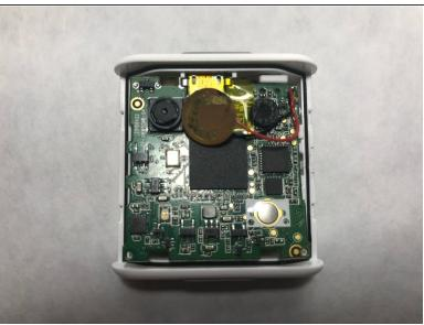
Use a nylon spudger to gently pry the four tabs holding the motherboard in place.
