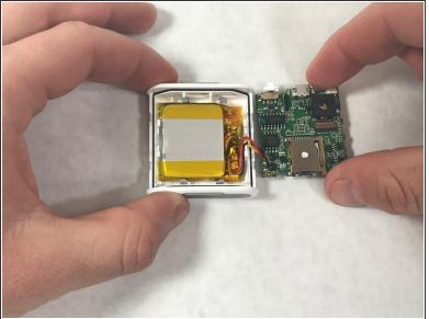
Lift the motherboard to reveal the battery compartment. Remove the thermal tape holding it in place and replace battery.
