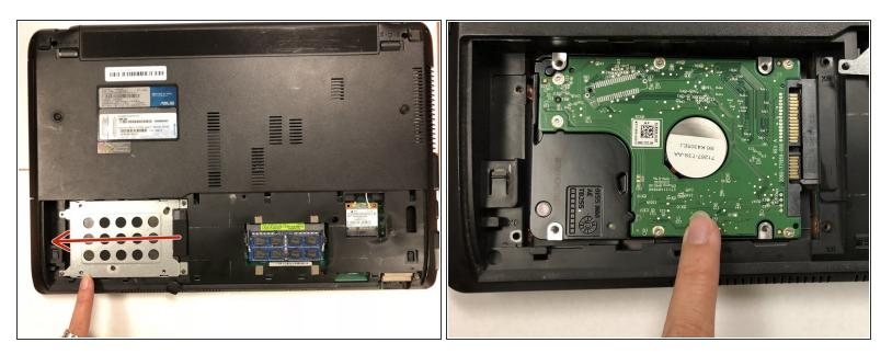
• Remove the silver hard drive cover by sliding it left to reveal the green hard drive.
