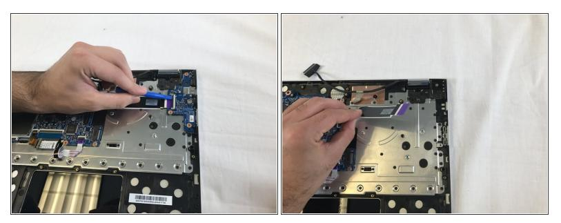
Use the plastic opening tool to open the security connector. then pull the ribbon cable to disconnect it from the motherboard.
