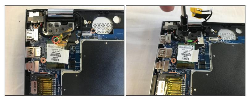
Use a PH0 tool bit to remove the one 2.8mm screw.
