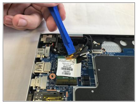
Use the plastic opening tool to disconnect Disconnect the two cables attached to the wifi
