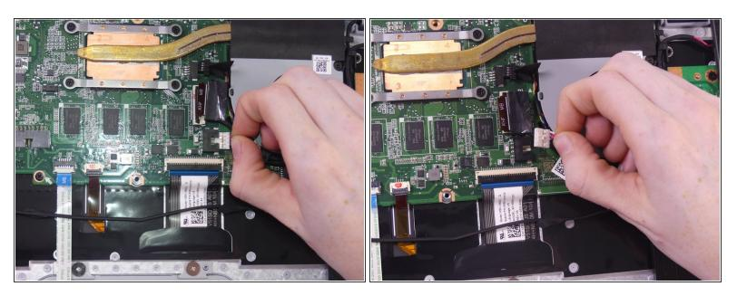
Remove the headphone jack wire by pulling it out of the connector socket.
