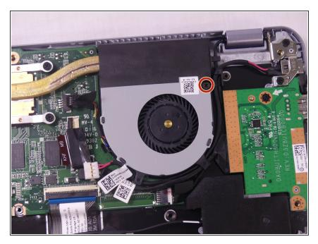
Remove the Phillip 3.6 mm screw from the fan using a Phillips #1 screwdriver.
