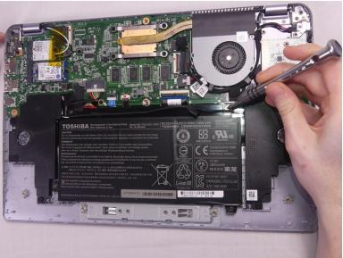
• Remove the 4 Phillips 3.2 mm screws holding the battery in place, with the Phillips #1 screwdriver.
