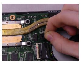
• The top wire is the fan's wire. Remove it by pulling it from the motherboard.
