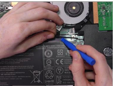
Remove the tape holding the speaker wire to the battery on both sides using a small opening tool.
