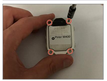
Use the T5 head on the iFixit screwdriver to unscrew the four screws on the back of the watch's face.
