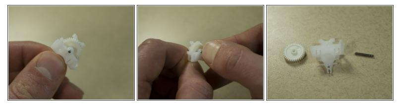
• Use your thumbnail and a pair of needle nose pliers to push out the gear housing retention pin.
