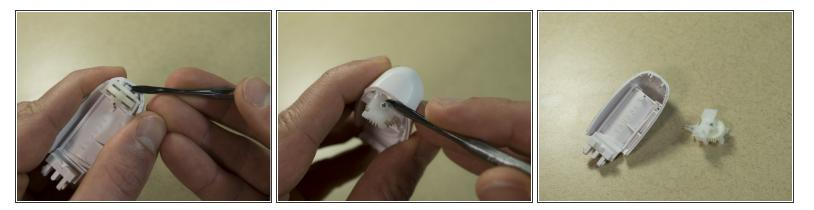
• Use a spudger to pry the gear housing unit from the base.
