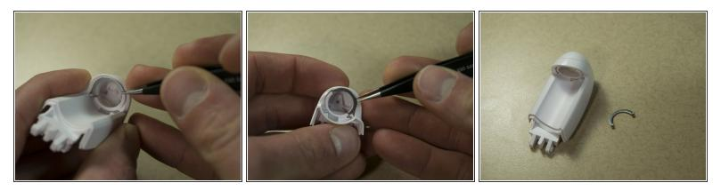
• Using Needle Nose pliers remove metal roller track on both sides of the Tweezers Head.
